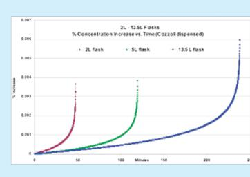
Thermal expansion will affect volumetric accuracy of calibrated flasks
