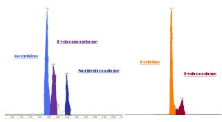
Figure 4: Chromatography of the Isobars (m/z 286 and 300, respectively)
