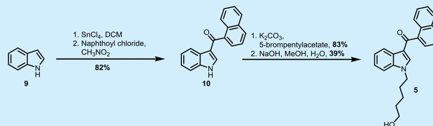
SnCl<sub>4</sub> acylation yield was 82% vs. 20% using Et<sub>2</sub>AlCl and 10% using MeMgBr
